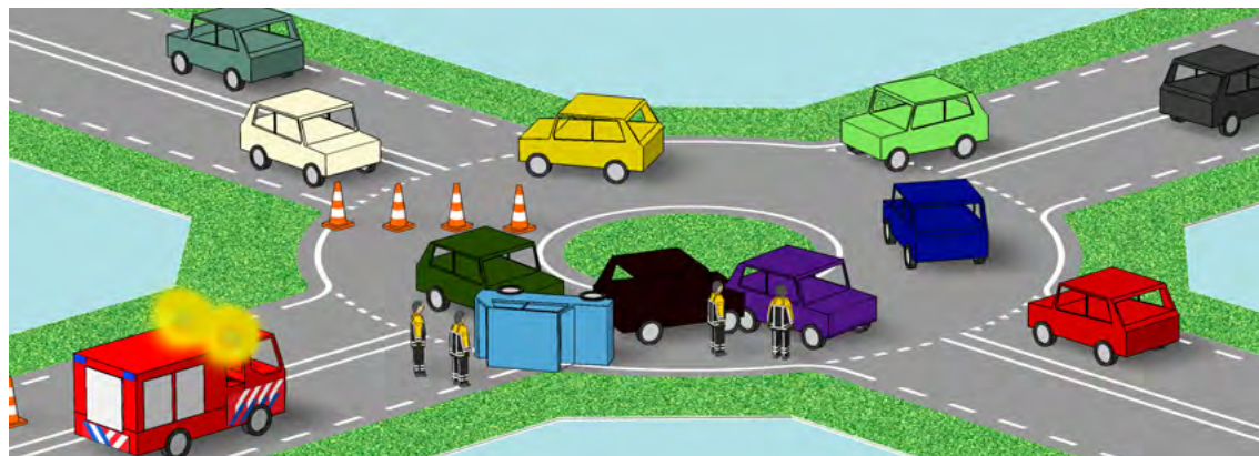
2 If the incident blocks access to the roundabout, the initial safety measures look like this.
