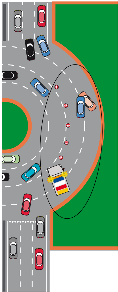
Figure a The incident in lanes 3 and 4 are protected by an emergency vehicle in fend-off position. The length of the safety zone is determined by the entry road ahead.
